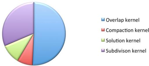
**Fig. 10.** The breakdown of the timings for the core of SST. Compute overlap kernel: 50.7%, Compaction kernel: 7.9%, Newton kernel: 10%, Subdivision kernel: 31.4%.
