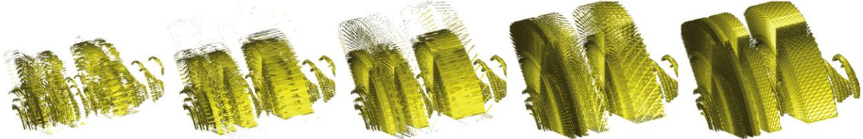
**Fig. 9.** Different isosurface snapshots rendering the velocity magnitude of air moving around a wind blade. The dataset consists of 800 K tri-quadratic rational Bézier patches ( $\approx 330$  MB).
