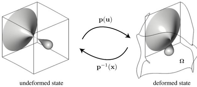
**Fig. 3.** Nonlinear deformation of a tri-quintic Bézier volume. The map also deforms an isosurface of an embedded scalar field. The inverse  $\mathbf{p}^{-1}(\mathbf{x})$  is highly nonlinear.
