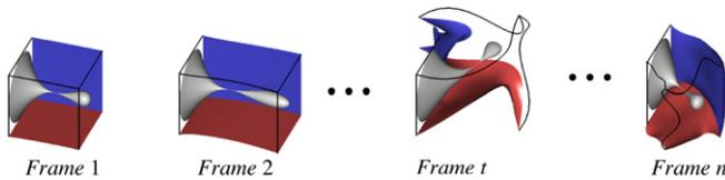
**Fig. 1.** Deformation sequence of an isosurface of a tri-quintic algebraic function. Methods to extract the implicit surface, such as Marching Cubes, are challenged because of the nonlinear distortions and thin surface features.
