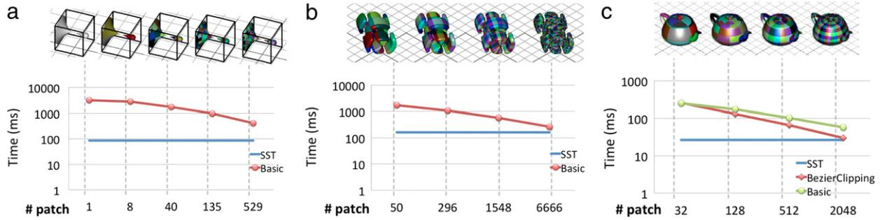
Fig. 12. The performance with respect to the number of patches for (a) teardrop, (b) cylinder, and (c) teapot.
