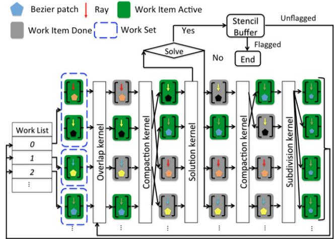
Fig. 6. Illustration of the SST core execution kernels.
