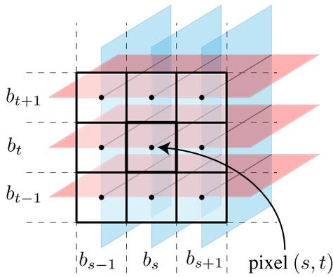
**Fig. 4.**  $3 \times 3$  pixel neighborhood on the near plane. Planes (red and blue) whose intersections coincide with pixel centers are defined as geometric constraints. (For interpretation of the references to colour in this figure legend, the reader is referred to the web version of this article.)
